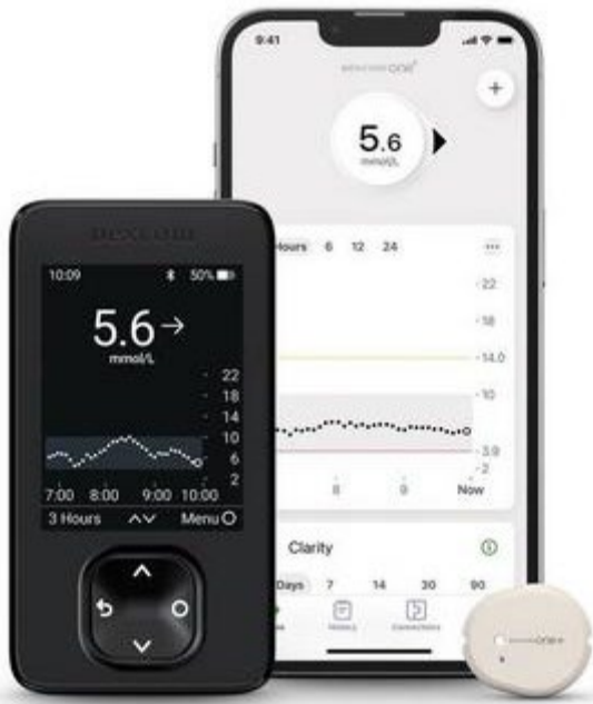
Figure 4 Dexcom ONE+ optional receiver, app display on a smart phone, and all-in-one transmitter and sensor
